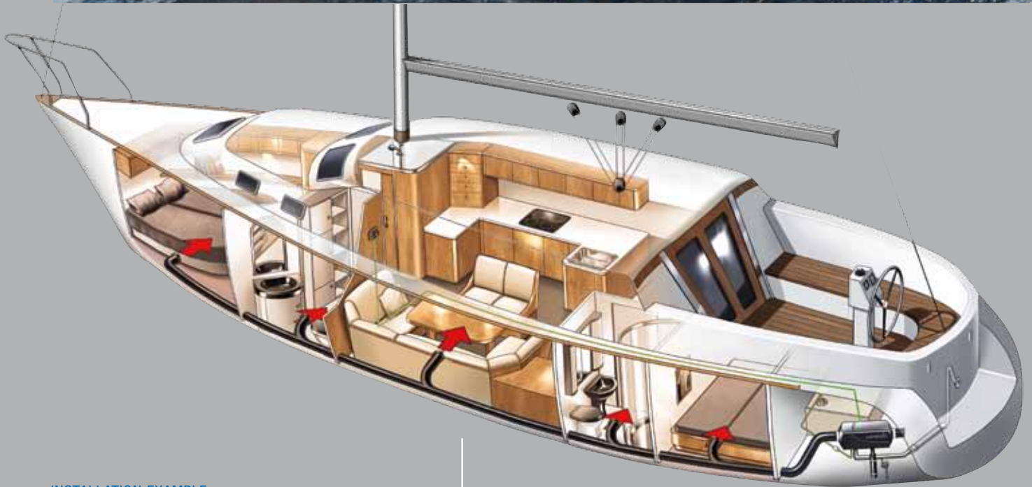
INSTALLATION EXAMPLE: Airtronic D4 in a 38-foot yacht.
