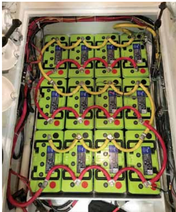
Firefly AGM batteries provide more battery capacity in less space, at a price.
